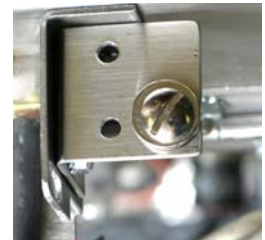
Figure 1: A cross-brace mounted bracket holds a switch and a tilt-plate mounted bracket holds the magnet in the new switch arrangement.
