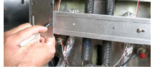
Figures 3 & 4: The outside holes of the far left bracket are aligned with the press studs (see arrows above) and the right side of the left bracket is marked for drilling additional mounting holes (see below).
